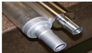
Formed Tube and Machined tube
